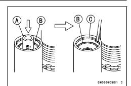
• Pull the gas reservoir cap [B] out of the gas reservoir using the pliers [A].
