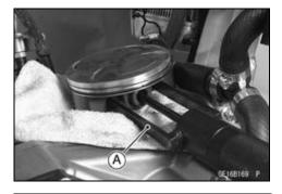
• Carefully spread the ring opening with your thumbs and then push up on the opposite side of the ring [A] to remove  $(\mathbf{A})$ Remove the oil ring in the same procedure.
