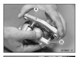
• Using compressed air, remove the pistons. One way to remove the pistons is as follows.
