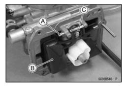
Bend the tang [A] on the float arm very slightly to change the float height. Increasing the float height lowers the fuel level and decreasing the float height raises the fuel level.
