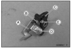
Set up the acceleration pump lever assembly as shown. Acceleration pump lever [A] Spring [B] Push Rod Holder [C]
