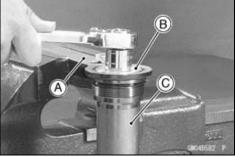
• Remove the base valve assembly [A] from the subtank [B].
