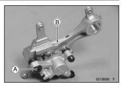
• Using compressed air, remove the piston.
