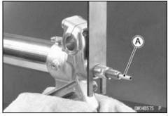
• With the outer tube compressed by hands, remove the top plug wrench [A].
