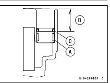
• Next, press the outside release shaft needle bearing [A] until the surface of the bearing is even with the crankcase surface [B].
