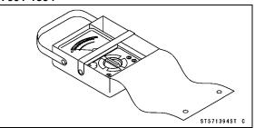
Throttle position sensor Setting Adapter #1: 57001-1400
