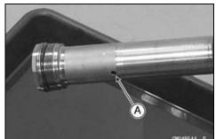
Compress the outer tube by hands and install the top plug wrench [A] between the axle holder bottom and locknut.
