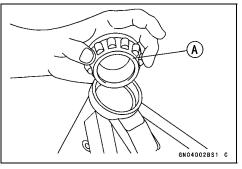
• Drive out the bearing outer races from the head pipe. ORemove the outer races pressed into the head pipe, using the head pipe outer race remover [A], and hammer the head pipe outer race remover to drive it out.
