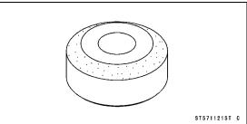
Valve Seat Cutter, 32° -  $\phi$ 38.5: 57001-1122
