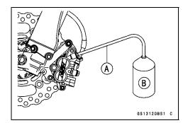
• Attach a clear plastic hose [A] to the bleed valve on the caliper, and run the other end of the hose into a container [B].
