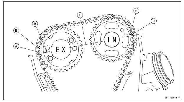
1st Pin [A] 2nd Pin [B] 29th Pin [C] Mark (exhaust) [D] Punch Mark (intake) [E] Upper Cylinder Head Surface [F]
