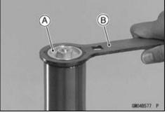
Remove: Cylinder Unit [A] Spacer [B] Fork Spring [C]
