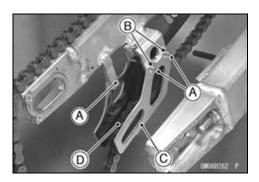
• Unscrew the rocker arm pivot nut [A] and pull out the rocker arm pivot bolt [B].
