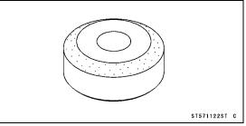
Valve Seat Cutter Holder,  $\phi$ 5.5: 57001-1125
