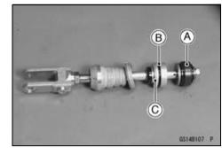
• Pry or tap [A] at the gaps [B] in the stop [C] with suitable tools to free the stop from the rear shock body [D].
