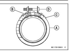
Torque - Carburetor Holder Clamp Screws: 2.0 N·m (0.20 kgf·m, 18 in·lb)
