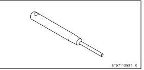
Valve Seat Cutter Holder Bar: 57001-1128
