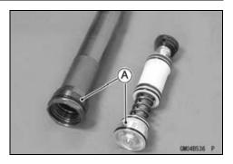
• With the piston rod in fully compressed position, pour the specified amount of fork oil [A].
