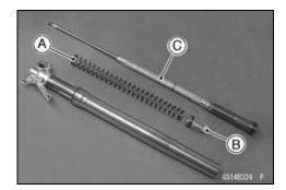
• Temporarily tighten the fork top plug [A] (subtank) using the top plug wrench.
