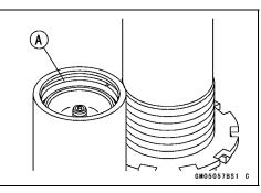
• Pull up the gas reservoir cap [A] against the circlip. The end of the gas reservoir cap must align [B] with the end of the gas reservoir [C].
