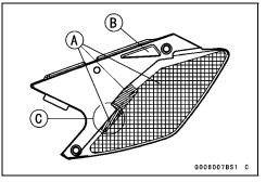
• Insert the tab [A] of the right side cover into the air cleaner housing [B], and install the bolts.
