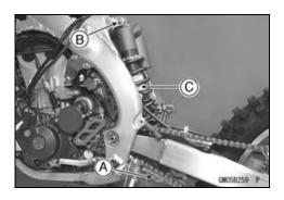
• Using the hook wrenches [C], loosen the locknut [B] and turn the adjusting nut [A] all way up.
