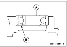
• Press the new drive shaft bearing [A] in the right crankcase [B] half, so that the stepped side [C] faces inside of the engine.
