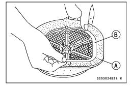
• Clean the element [A] in a bath of a high-flash point solvent using a soft bristle brush.
