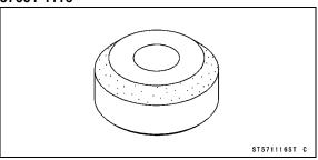
Valve Seat Cutter, 32° -  $\phi$ 35: 57001-1121
