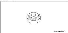
Valve Seat Cutter, 55° -  $\phi$ 38.5: 57001-1497
