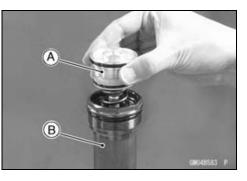
• Drain the fork oil [A] from the cylinder unit [B] by pumping the piston rod several times.
