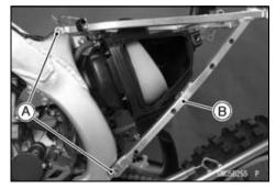
• Using the hook wrenches [A], loosen the locknut [B] on the rear shock absorber.
